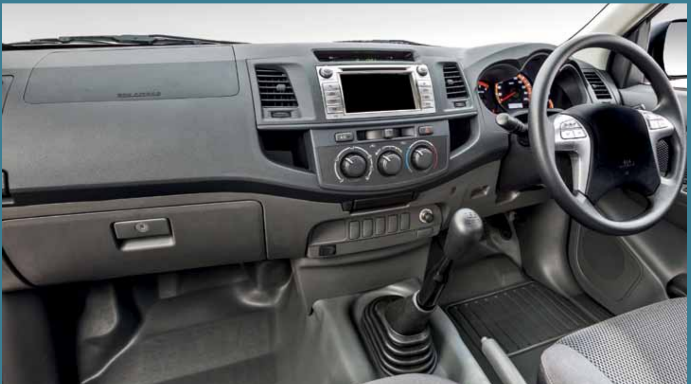
Examples of instrument panels in car vehicles that utilize impact-resistant copolymer resin in its manufacture.
